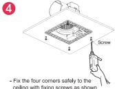
ceiling with fixing screws as shown in the figure.
