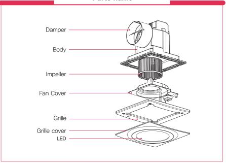
The surroundings of fan and grille are easily stained with dust or smokes, so they should be cleaned regularly every  $2\sim3$  months.
