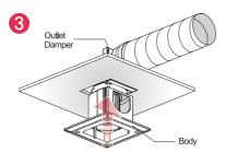
Insert the body to the top in the direction of the arrow to fit the guide of the damper.
